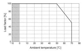
Specifications for ripple and ripple noise changes in the shadedarea.
