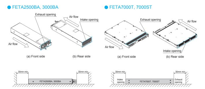
When mounting the power supply with screws, it is recommended that this be done as shown in below figure. If other methods are used, be sure the weight of the power supply is taken into account.
